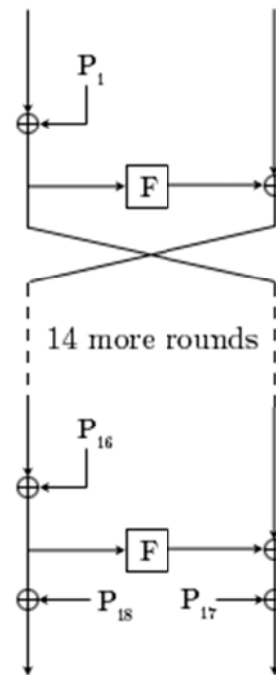
The Feistel structure of Blowfish
